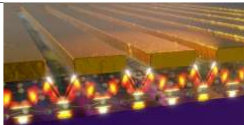
Figure 1: Schematic of the 2D polaritonic nanoresonator that show the field intensity of the propagating mode.
