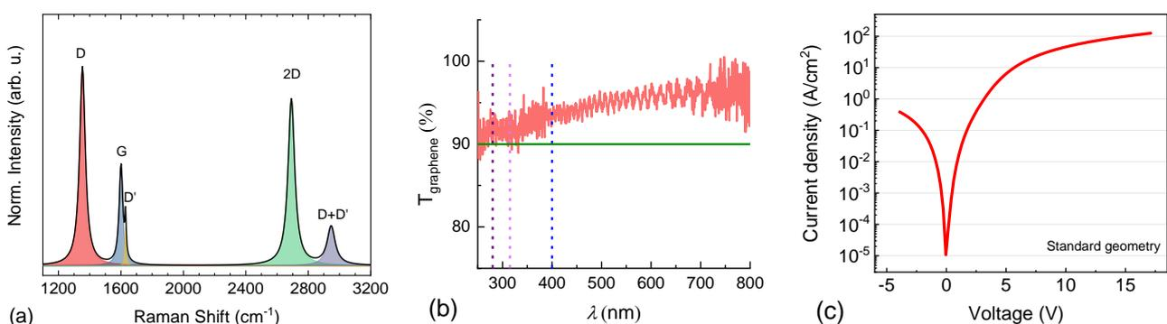
**Figure 1:** (a) RAMAN spectrum and (b) transparency of PECVD as-grown graphene on p-Al<sub>x</sub>Ga<sub>1-x</sub>N. (c) Current density vs. voltage of a graphene enhanced UV LED in standard geometry.
