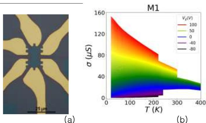
**Figure 1:** (a) Optical picture of a monolayer MoS<sub>2</sub> Hall bar (M1). (b) Four-probe conductivity of a device showing a MIT around  $V_g=45\text{V}$ .
