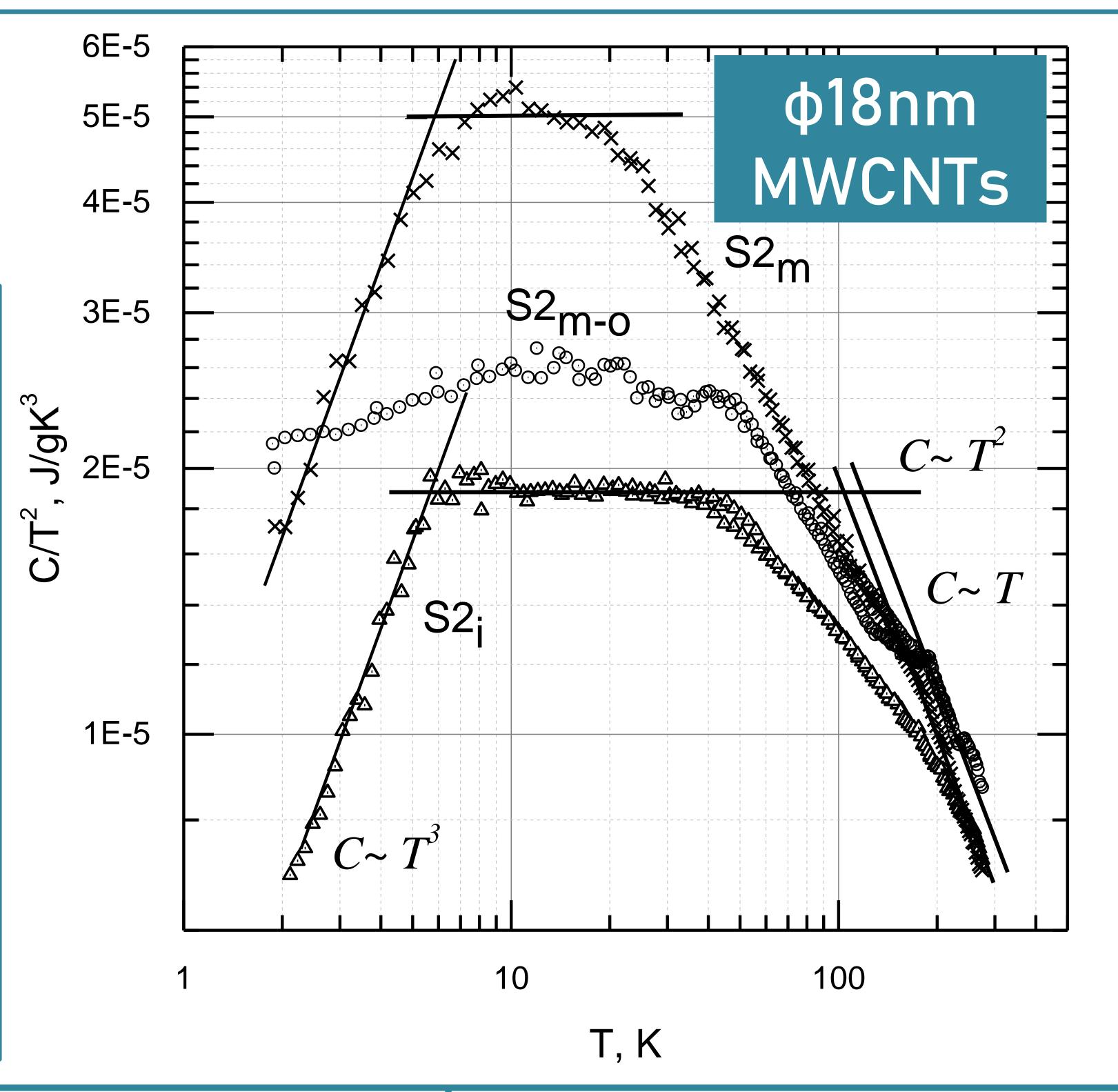
The parameters of defects change and their number increases during the grinding of oxidized MWCNTs Ø7.2 nm and Ø18 nm. As a result the increase of the phonon density of states in the low-energy part of the spectrum and, correspondingly, an increase of the heat capacity of nanotubes of Ø7.2 nm and Ø18 nm can occur.
