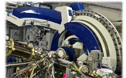
Diffractometer + MBE chamber @BM32
