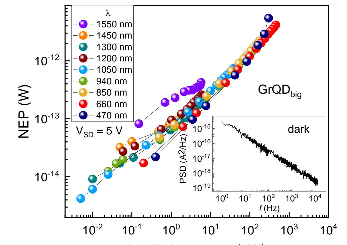
□  $\text{NEP} = 4 \times 10^{-15} \text{ W}$  for integrated noise PSD,  $7 \times 10^{-15} \text{ A}^2/\text{Hz}$
