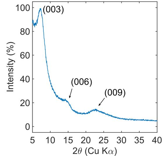
X-ray diffraction pattern of citrate containing NiFe-LDH dispersion drop-casted on Si(100).
