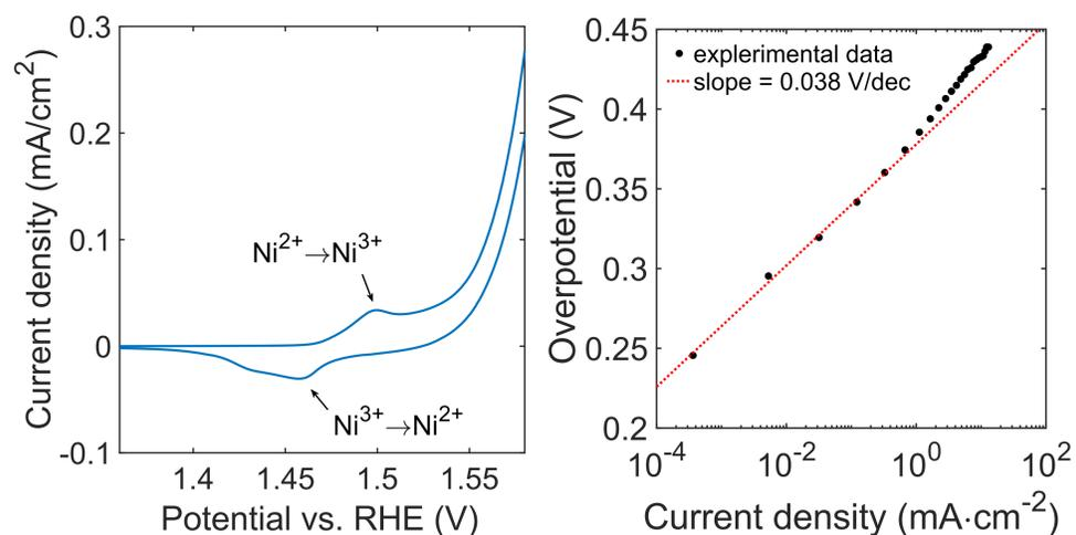
The polarization curve of NiFe-LDH nanosheets deposited on carbon paper shows an electrocatalytic activity for the oxygen evolution reaction (OER). We measured an overpotential of 0.43 V @ 10 mA/cm<sup>2</sup> current density with a mass loading 0.1 mg/cm<sup>2</sup>. Moreover, a Tafel slope of 38 mV/dec is retained for current densities up to 10 mA/cm<sup>2</sup>.
