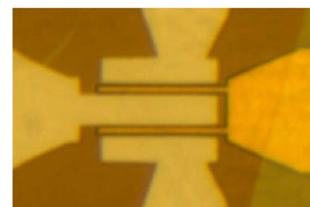
Optical image of the RF GFET on hBN with buried bottom gates
