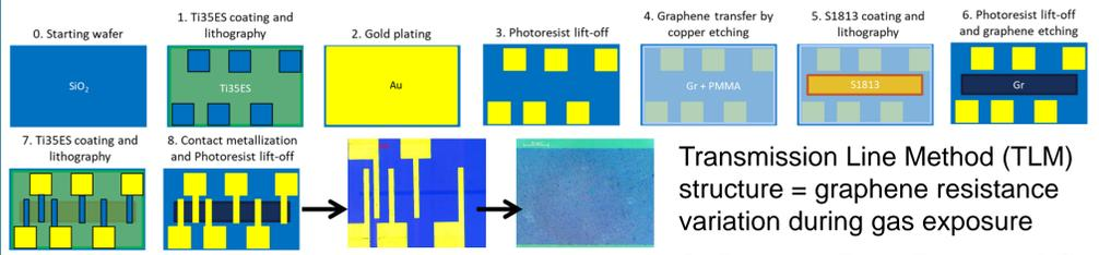
Transmission Line Method (TLM) structure = graphene resistance variation during gas exposure
