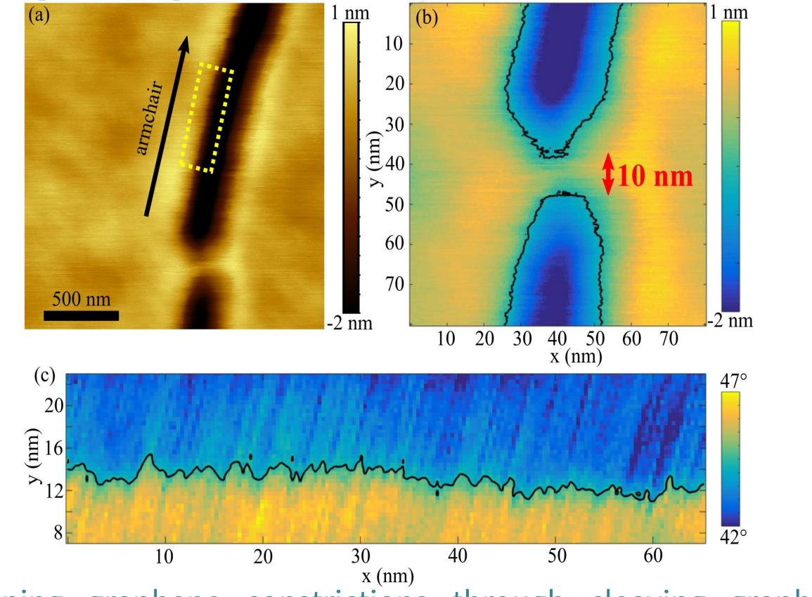
Defining graphene constrictions through cleaving graphene sheets by AFM along their high symmetry directions, enables us to fabricate graphene nanoconstrictions down to 10 nm width and with reduced edge roughness of +/- 1 nm. The quality of the edges is preserved, since constriction edges never come into contact with resist material or wet chemistry.
