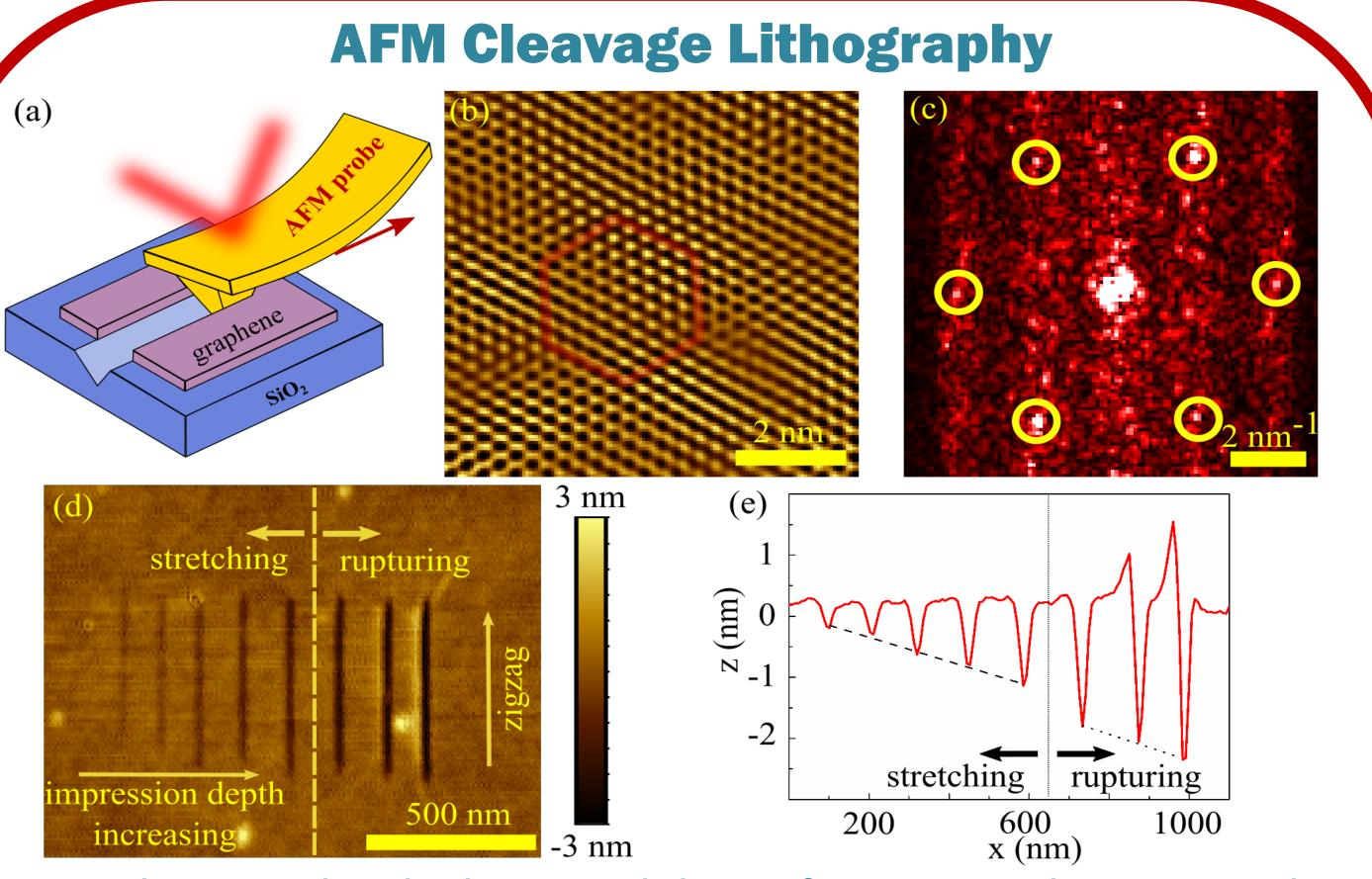
We have utilized the capability of AFM to determine the crystallographic orientations of the graphene lattice before patterning. This made it possible to cleave graphene sheets along their high symmetry directions. After reaching a critical indentation depth, the chances of graphene rupture increase dramatically. Despite the smooth edges, on a series of test lines the two regions can be distinguished.
