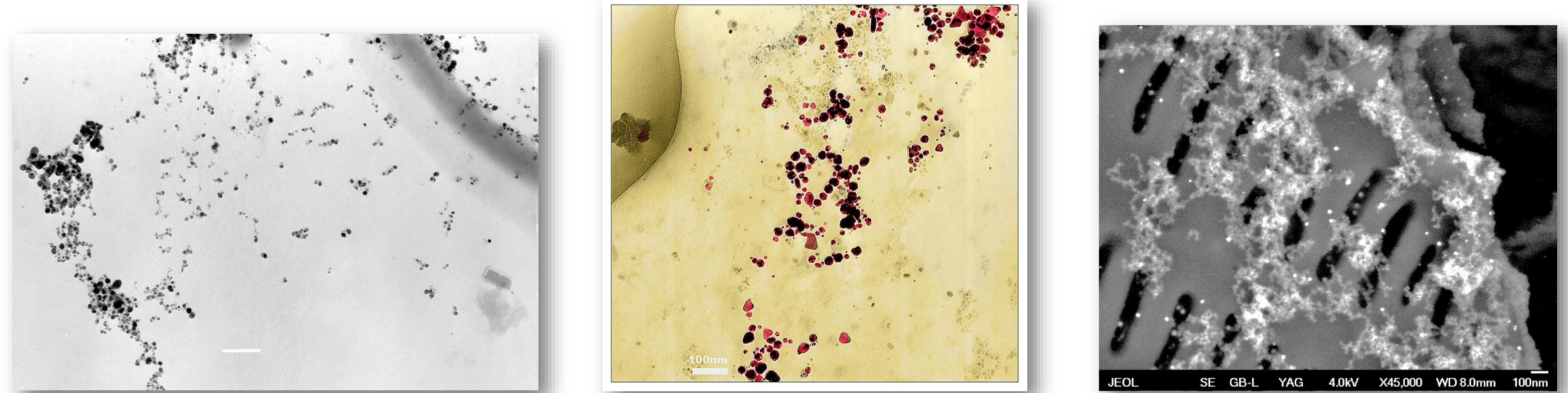
Left – Ag NP reduced and stabilized by Anabaena mendotae , Middle - Mallomonas kalinae with AuNP (colored in Photoshop), Right - Au NP reduced on the Diademsis gallica siliceous frustule, modified with ferrofluid (scale 100 nm)
