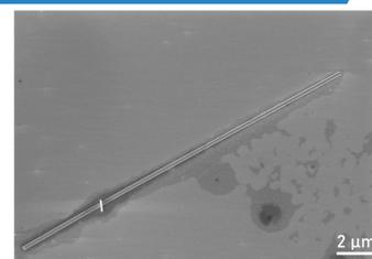
Fig. 7: Typical SEM image of a dropcasted NR
