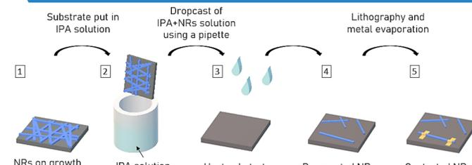
Fig. 6: Schematic of the different steps involved in the sample preparation for electrical characterization.
