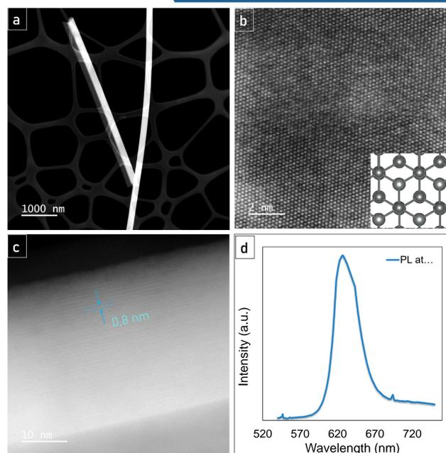
Fig. 5: (a) STEM observation of dropcasted NRs on TEM membrane. (b) High magnification TEM image of the center of a nanoribbon. (c) High magnification TEM image of a NT. Inter-layer spacing measured to be 0.8 nm. (d) PL spectrum of several NRs
