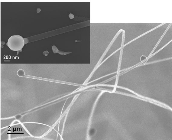
Fig. 4: SEM images of as-grown NRs. In inset, a high magnification image shows the droplet sitting on top of a NR
