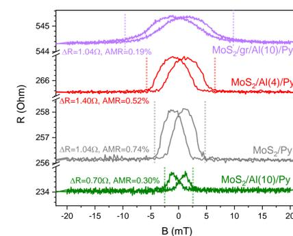
**AMR measured** by applying a DC current of 50  $\mu A$  and sweeping the magnetic field  $B$  in the sample plane and perpendicular to the current direction.
