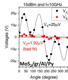
Symmetric and antisymmetric voltages ( $V_S$  and  $V_A$ , respectively) are extracted from ST-FMR curves measured varying the angle between the current and the external magnetic field  $B$ .
