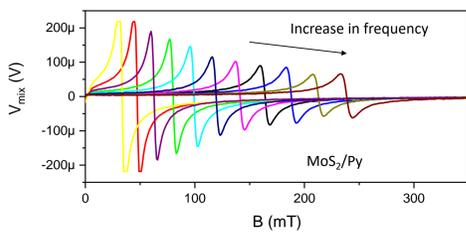
From measurements for **different frequencies** (GHz) of RF current (with a fixed angle between the current and the magnetic field) it is possible to extract the effective magnetization ( $M_{eff}$ ) and the Gilbert damping ( $\alpha$ ), as follows:
