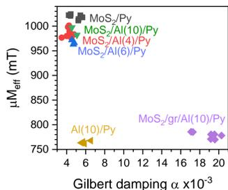
Extracted **effective magnetizations** show a striking difference between samples with MoS<sub>2</sub> and samples without MoS<sub>2</sub> or with graphene spacer.
