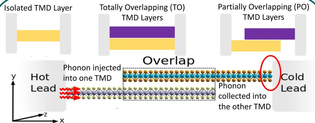
Previous electronic characterizations (theoretical [2] and experiments [3-4]) showed that such setups favour inter-layer band-to-band tunnelling and can therefore be used as field-effect transistors with a potentially steep subthreshold swing and a high ON-state current.
