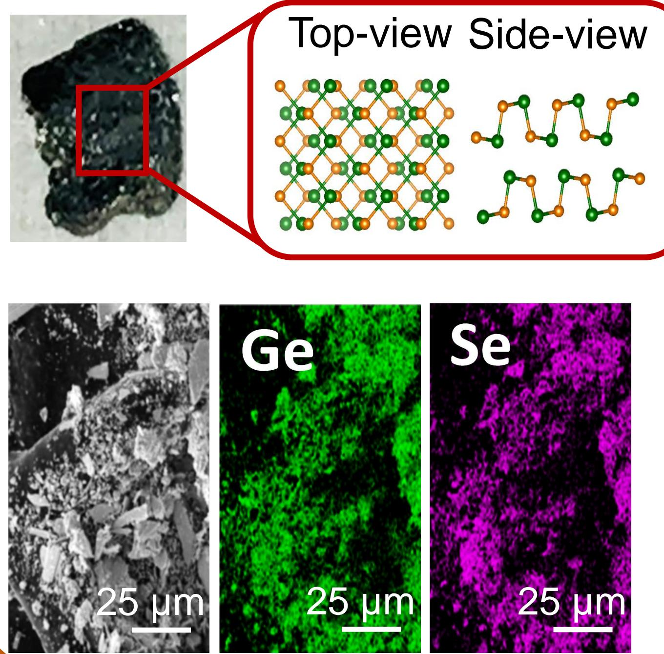
Depending on pH and thickness, GeSe nanoflakes can act as photocatalysts for hydrogen and oxygen evolution reaction (HER) and OER).
