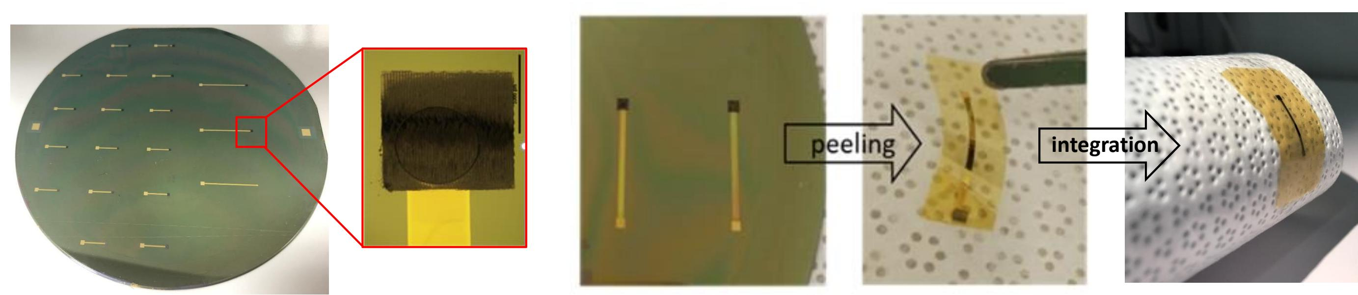
Thermal annealing at 350°C during 8 h after fabrication
