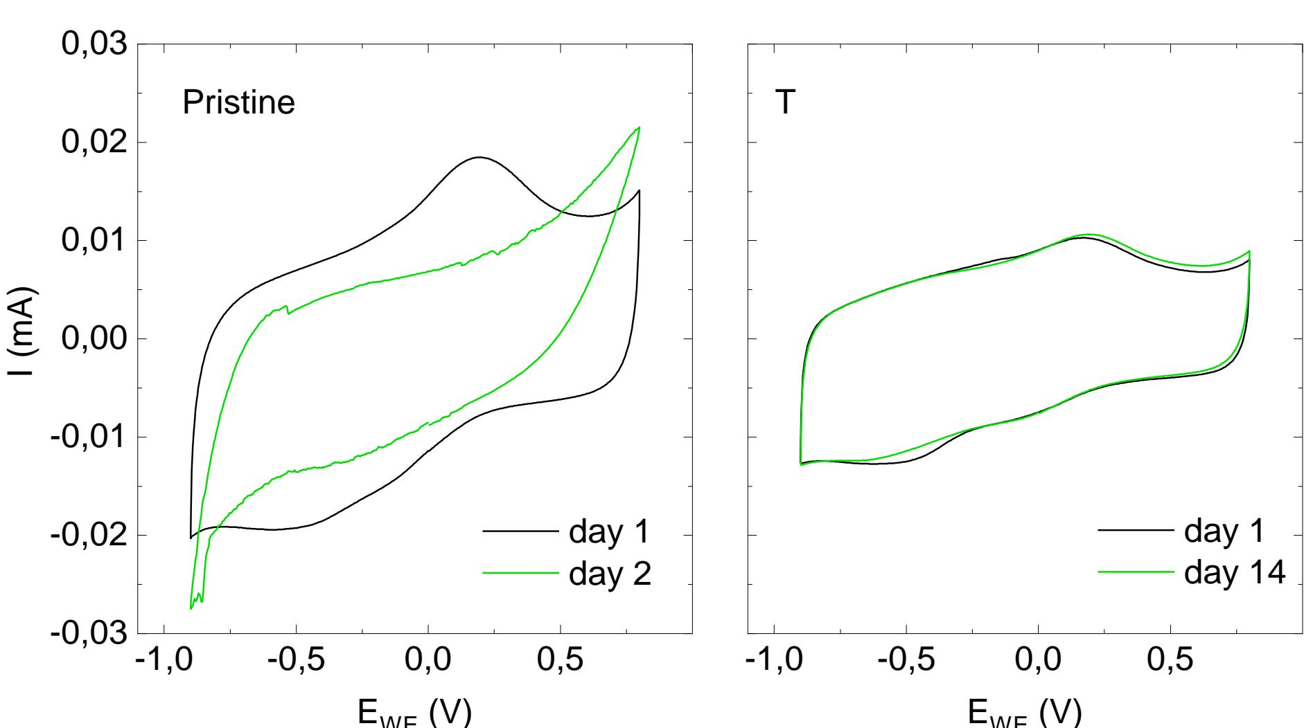
1. Thermal annealing process increases the electrode stability. Before the thermal annealing treatment, electrode needs different cycles to be more stable
