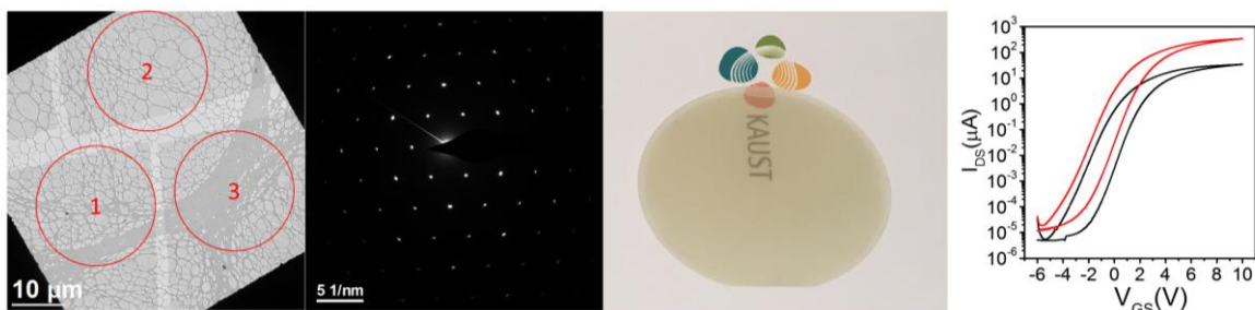
Figure 2: wafer-scale single-crystalline MoS 2 films with high electric performance
