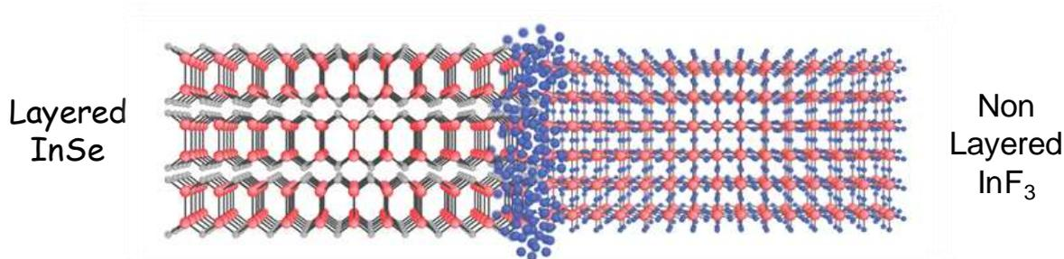
**Figure 1:** Schematic showing chemical conversion of 2D InSe to InF<sub>3</sub> nanosheets.
