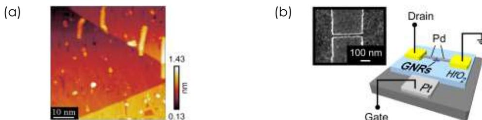
**Figure 2:** (a) Scanning tunnelling microscope image of nanoribbons used for transistors. (b) Schematic diagram of GNR-transistor device structure. The inset shows the SEM image of the Pd nano-gap.
