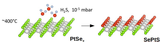
Figure: Schematic of the sulfurization process (annealing in H 2 S gas pressure) by which SL PtSe 2 is transformed into a Janus SePtS compound.
