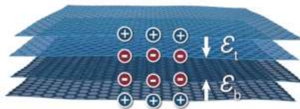
Figure 1: Crystal fields in twisted double bilayer graphene lead to the spontaneous opening of a band gap
