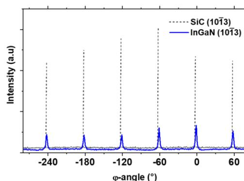
**Figure 2:** XRD  $\phi$ -scan performed on the (10 $\bar{1}$ 3) reflection of the InGaN (blue curve) and the 6H-SiC (black dashed curve) substrate showing their epitaxial relationship.
