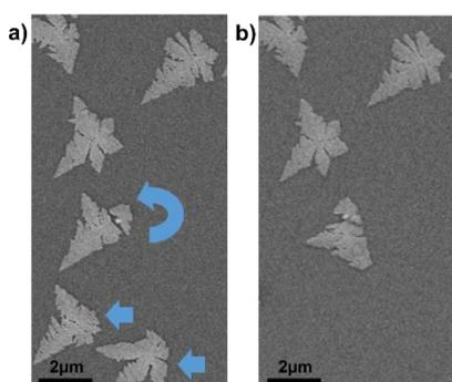
**Figure 1:** SEM images of InGaN islands on graphene (a) before and (b) after local AFM scanning in contact mode of the bottom part of the image. The blue arrows show the displacement of the nuclei confirming their weak bonding with the substrate.
