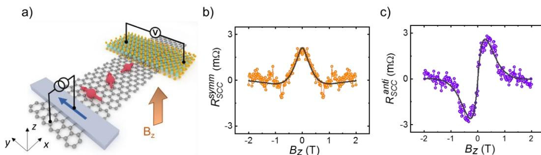
**Figure 1:** (a) Schematic of the measurement configuration showing the spin precession by applying an out-of-plane magnetic field. (b-c) Symmetric and antisymmetric components of the spin-to-charge conversion signal fitted to the Bloch equation (solid black line) corresponding to the spin to charge conversion of the spin component along y and x directions respectively.
