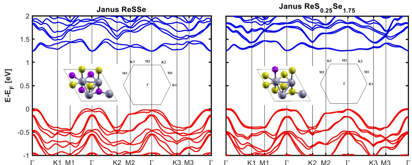
**Figure 1:** Left: Band structure plot for Janus ReSSe along special symmetry points, as marked in the figure of the Brillouin zone in the inset. Right: Band structure plot for Janus ReS<sub>0.25</sub>Se<sub>1.75</sub> along special symmetry points, as marked in the inset. The figure in the inset of the graphs show the unit cell of the Janus monolayer, with Re in grey, S in purple and Se in yellow.
