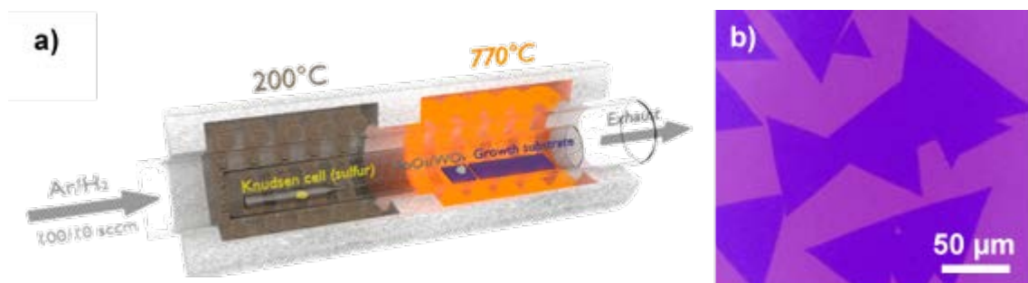
Figure 1: a) Scheme of the CVD growth system. b) Optical microscopy image of monolayer crystals of MoS 2 .
