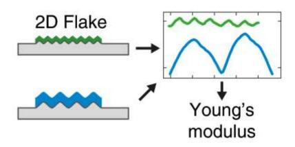
**Figure 1:** The spontaneous formation of periodic wrinkles is due to the buckling instability that occurs in thin 2D flakes deposited onto a prestrained relatively soft, thick substrate. Using the spacing of the periodic wrinkles one can calculate the 2D material in-plane elastic modulus by applying well-established buckling mechanics equations.
