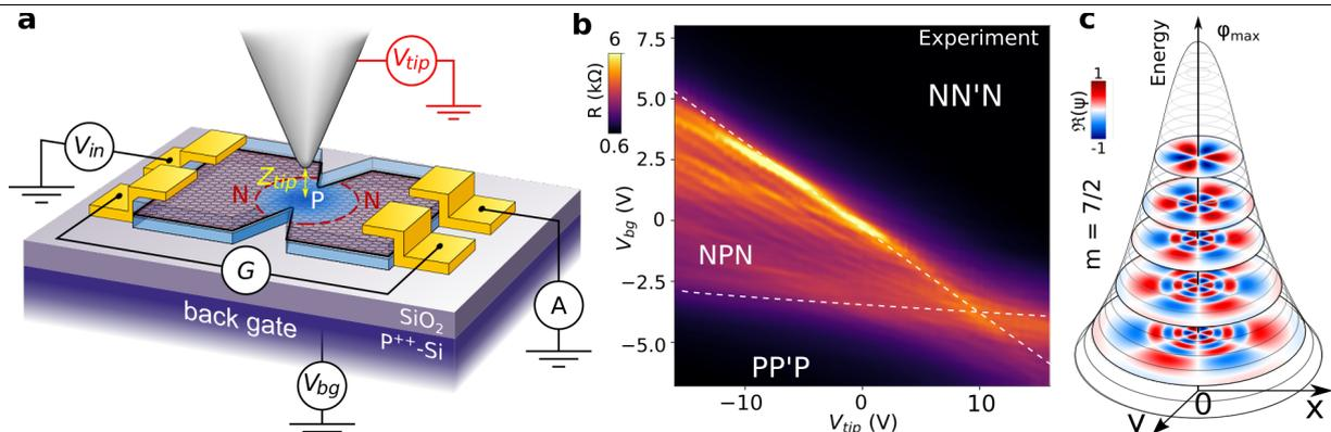
Figure 1: **a**, Scheme of the experiment: a polarized AFM tip is scanned above a constriction etched in an encapsulated graphene device. **b**, Resistance of the device as a function of tip and backgate voltages, when the tip is placed above the center of the constriction. **c**, Wave function corresponding to the WGM with angular momentum  $m = 7/2$ , for its different resonant energies.
