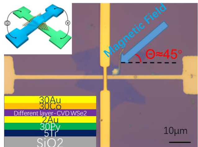
Figure 1: Device structure & measurement method
