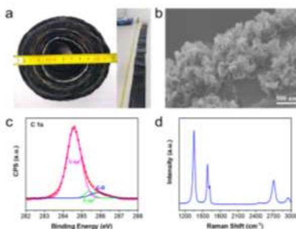
**Figure 1:** (a) Optical photos of hierarchical graphene functionalized Al foil (hG-Al foil) by CVD batch preparation; (b) SEM image of hierarchical graphene structure; (c) XPS C-1s spectrum of hG-Al foil; (d) Typical Raman spectrum of hG-Al foil.
