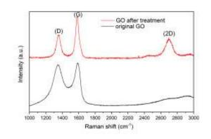
Figure 1: Raman spectra of original GO and GO after thermite treatment.
