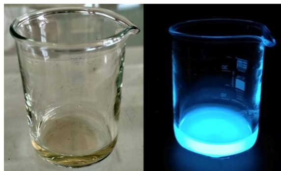
Figure 1: Photoluminescence of NH 2 -CNPs under UV light (365 nm)
