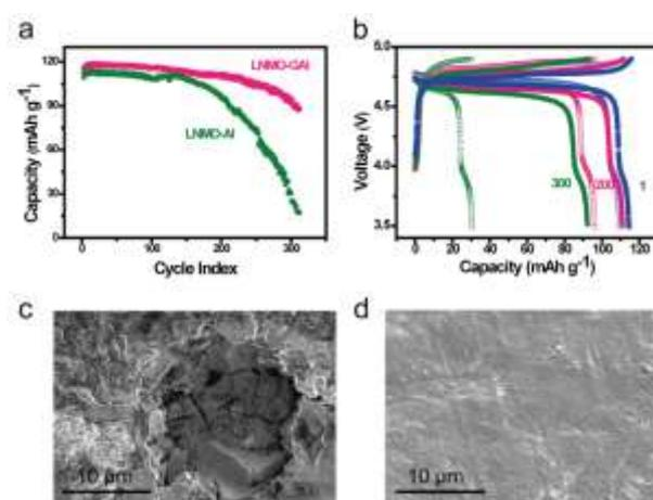
**Figure 1:** Enhanced anticorrosion performance of GAI. (a,b) Long-term cycling performance of LNMO/GAI and LNMO/Al cells; (c, d) SEM images of pristine Al foil and GAI after cycling;
