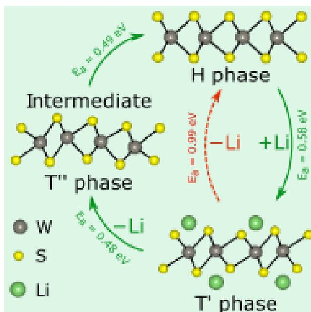
**Figure 1:** Flow diagram for transition of WS<sub>2</sub> showing the reverse conversion via an intermediate mixed phase
