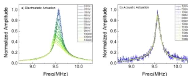
**Figure 2:** Frequency sweeps for a) Electrostatic and b) Acoustic actuation of graphene membrane as a function of increasing ac drive force. The y-axis denotes output amplitude divided by the driving amplitude.
