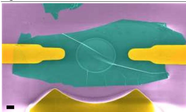
**Figure 1:** SEM image (false colors) of suspended multilayer graphene sheet on 10 $\mu$ m circular cavity. The AlN piezo-stack is also visible at the bottom of the image. The scale bar is 2 $\mu$ m.
