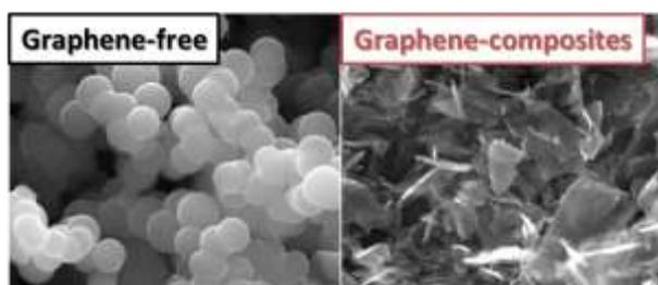
**Figure 1:** SEM images of graphene-free and graphene-composites
