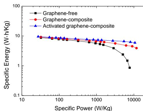
**Figure 2:** Ragone plot of graphene-free, graphene-composite and activated graphene-composite in the aqueous electrolyte 1M H<sub>2</sub>SO<sub>4</sub>
