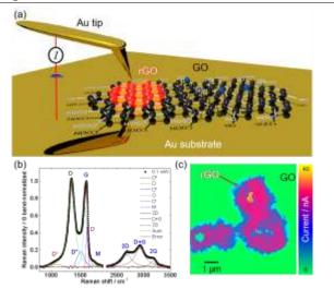
**Figure 1:** (a) Schematics of the laser patterning reduction of GO. (b) Raman and (c) One CSAFM result on GO film
