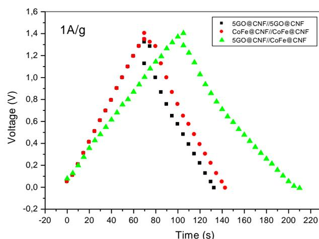
Figure 2: Galvanostatic charge/discharge curves of ASC.
