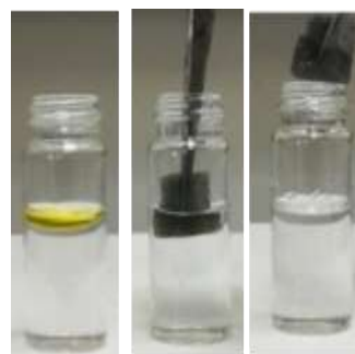
Figure 1: Digital photographs of: olive oil floating on water (left), a graphene-coated melamine foam adsorbing the oil phase (middle), and the final oil-free water after extraction of the sorbent (right).
