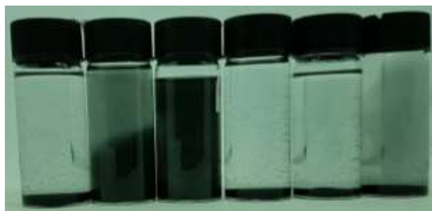
Figure 2: A photograph of graphene dispersions via radical stabilization
