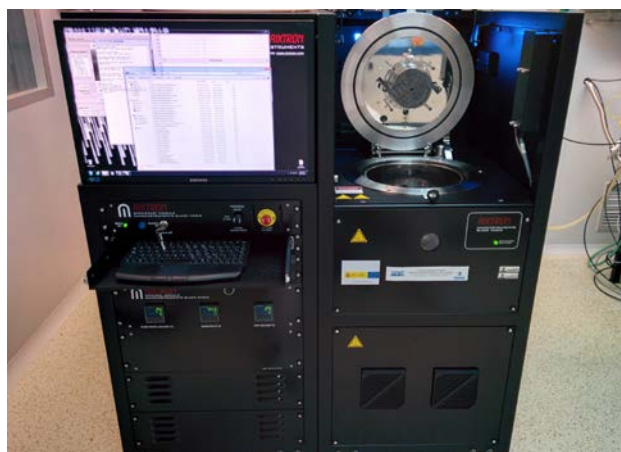
Figure 1: Cold-wall CVD reactor Aixtron BM Pro. In a typical growth, 4-inch graphene samples are grown in less than 2 hours.
