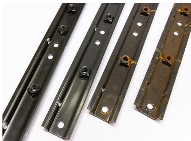
Figure 1: Scania Truck head lamp brackets ACT chamber 6 weeks, equivalent to 3y field use. Piece treated with GO to the left together with different non-GO coatings. Picture provided by Provexa AB.
