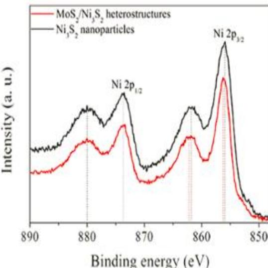
The XPS shifts strongly suggest the existence of **strong electronic interactions** between Ni<sub>3</sub>S<sub>2</sub> and MoS<sub>2</sub>, which implies the **establishment of coupling interfaces**.
