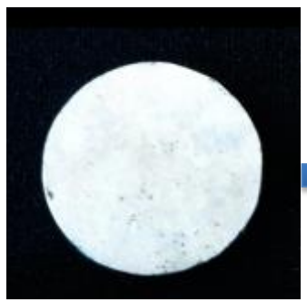
well-crystallized h-BN bulk sample (pellet)
