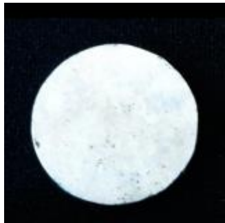
well-crystallized h-BN bulk sample (pellet)
