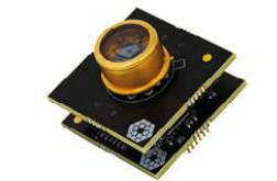
Analog component package for detector chip and TEC element
