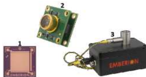
Figure 1: Emberion's single pixel photodetector device (1), photodetector module (2) and the evaluation kit for customer demonstrations (3)
