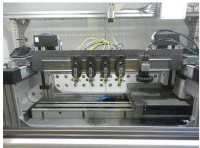
Figure 1: Multiple spray-gun deposition machine for nanomaterials (Graphene Flagship)
