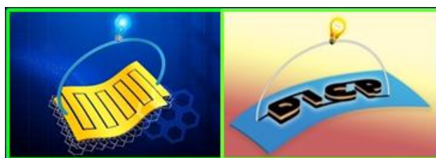
Figure 1: Graphene based interdigital planar MSCs (left) and arbitrary-shape sandwich planar MSCs (right)
