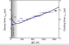
**Figure 2:** Comparison between measured decay time and calculated cooling time as a function of electron temperature. [7]
