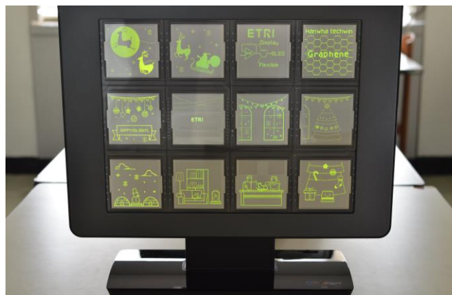
Figure 1: 370 mm×470 mm sized Graphene anode OLED panel with driving capacity.
