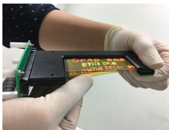
Figure 2: Flexible OLED with pixelated Graphene electrode array.
