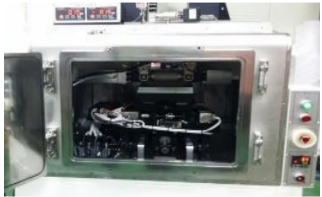
Figure 1: Vacuum transfer equipment
